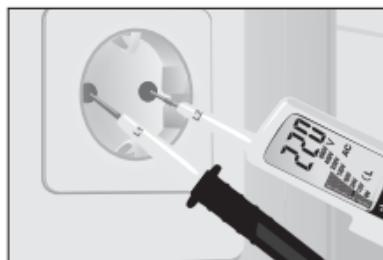
Hold the base device (+) in your right hand and the second test prod (-) in your left hand. Now apply the test prods to the contacts to be tested (line, socket, etc.).
