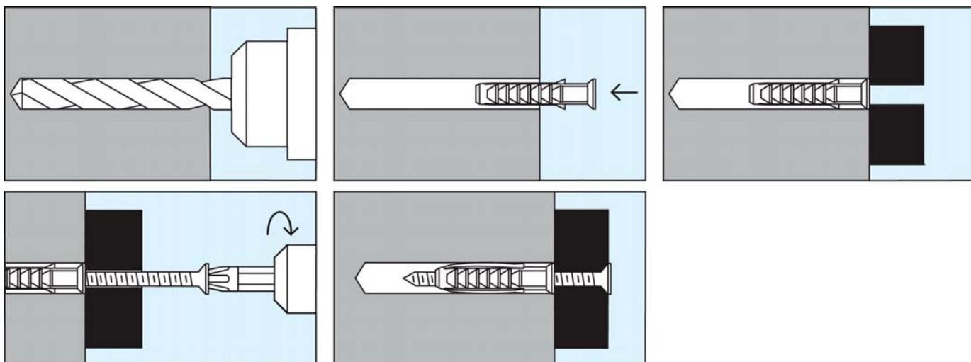
**SEQUENZA DI MONTAGGIO PER FISSAGGIO PASSANTE**
