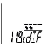
This mode refers to the infrared temperature and calculates the difference between the maximum and minimum infrared temperature while measuring. The value is deleted and calculated again at the start of a new measurement or by pressing the trigger (9).
